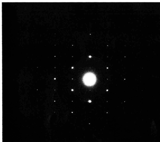
Fig. 2. An hk0 electron diffraction pattern from a multilayer crystal of DL-(1,2/3)-1,2-di-O-palmitoylcyclopentane-1,2,3-triol. The intensity distribution of the diffraction pattern can be compared to a monolayer type pattern by reference to Fig. 2 of Reference 6. Accelerating voltage: 100 kV. Subcell axes: a_s \cong 7.5 \text{ \AA} , b_s \cong 5.0 \text{ \AA} .
