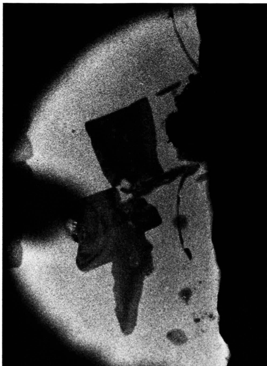
Fig. 5. Bright field diffraction contrast image of the crystal used to obtain the diffraction pattern in Fig. 2, the large dark area on the crystal surface, due to parts of the crystal in perfect Bragg incidence, indicate the crystal to be only slightly bent.
